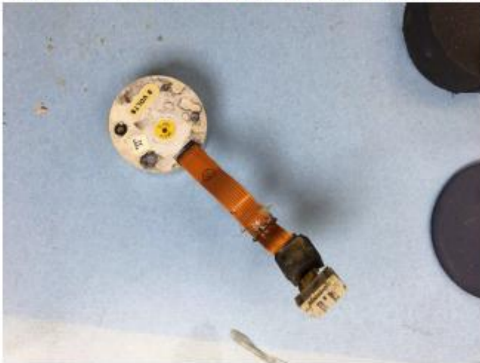
Figure 2. Extracted memory module showing discoloration from contact with salt water.
