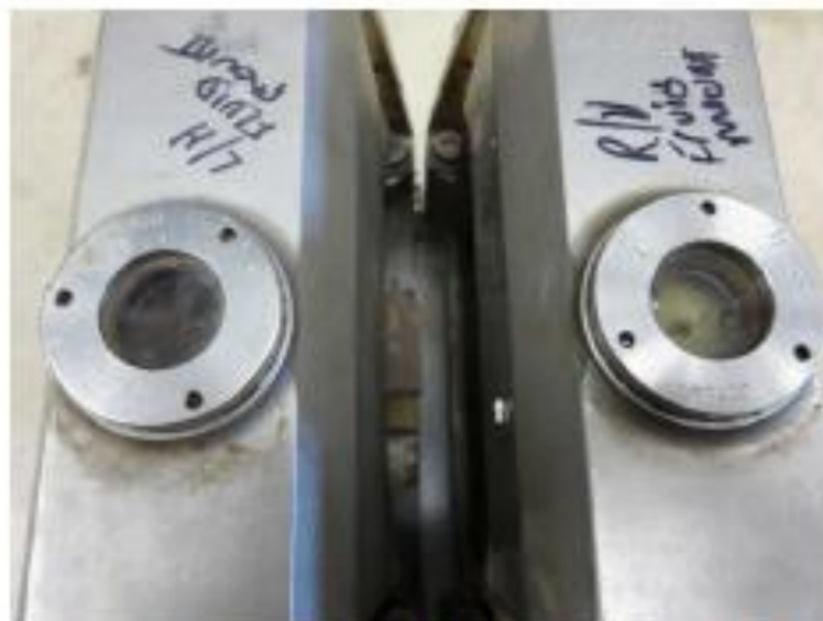
Figure 15: Overview of vertical pylon mounts (top image). Fluid was visible through the sight glass on the top of each mount (bottom image).
