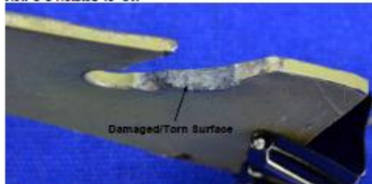
Figure 12: Representative condition of the torn screw holes on submitted skin/structural panel sections removed in the lab from the airframe components.
