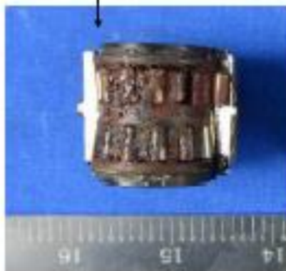
Figure 6: The Orange universal bearing was seized by corrosion products and no noticeable amount of grease was present on either end of the bearing. The Red universal bearing required atypically high and inconsistent torque to rotate, but had significantly less corrosion product and a noticeable amount of grease.
