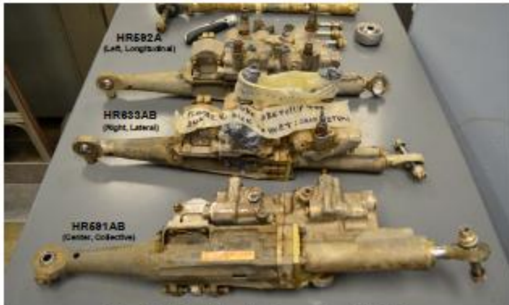
Figure 17: The hydraulic actuators as-received in the lab.
