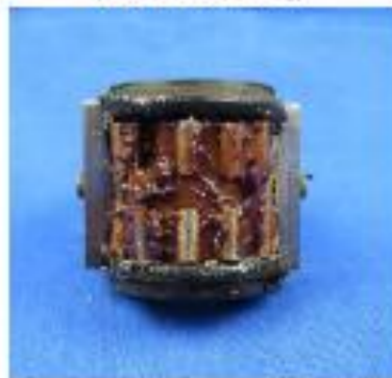
Figure 6: The Orange universal bearing was seized by corrosion products and no noticeable amount of grease was present on either end of the bearing. The Red universal bearing required atypically high and inconsistent torque to rotate, but had significantly less corrosion product and a noticeable amount of grease.
