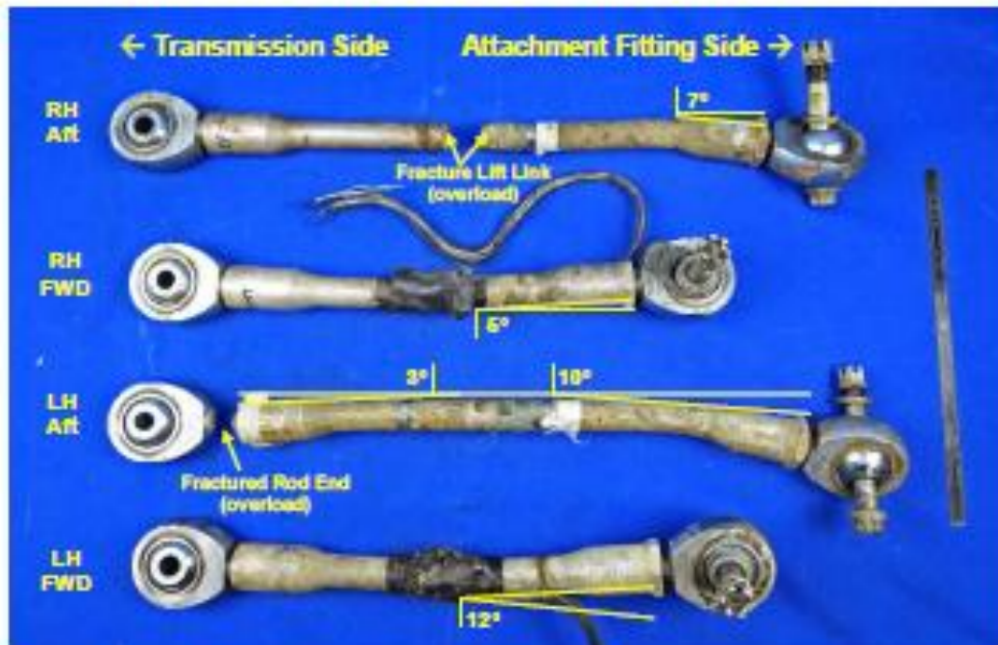
Figure 13: View of the bent lift links with the bend locations and angles provided. A view of the fractured rod end attached to the left-hand aft lift link is shown in Figure 14.
