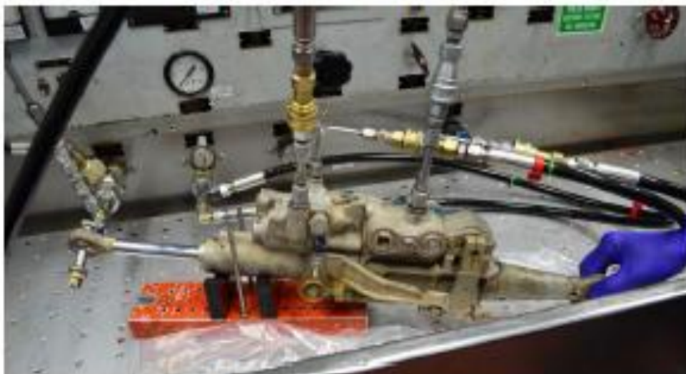
Figure 18: Setup used for hydraulic bench testing.
