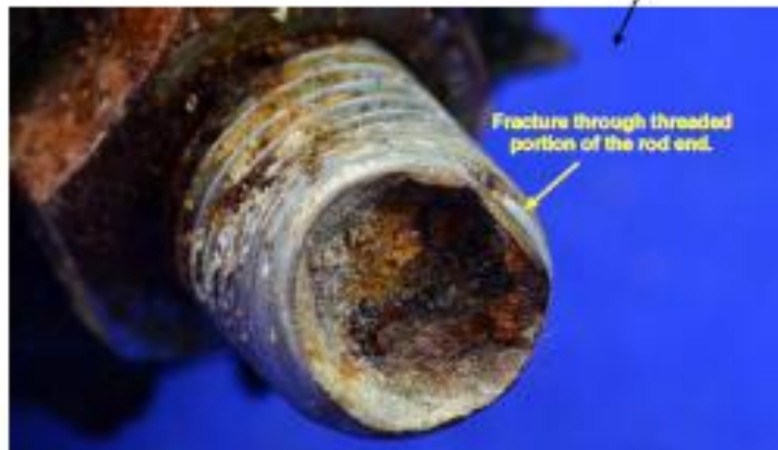
Figure 15: The threaded portion of the fore/aft restraint rod end was fractured. The ductile deformation and "cup and cone" features of the fracture are consistent with overload. The fracture face itself was heavily corroded.
