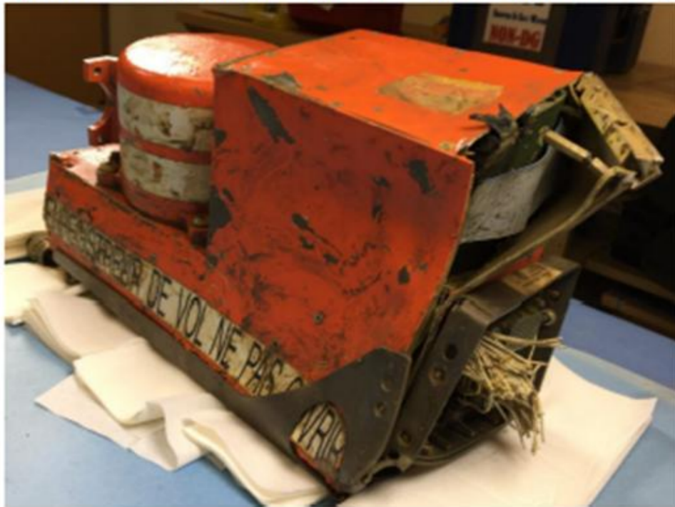
Figure 1. Exterior of flight recorder showing mechanical impact damage and broken casing.
