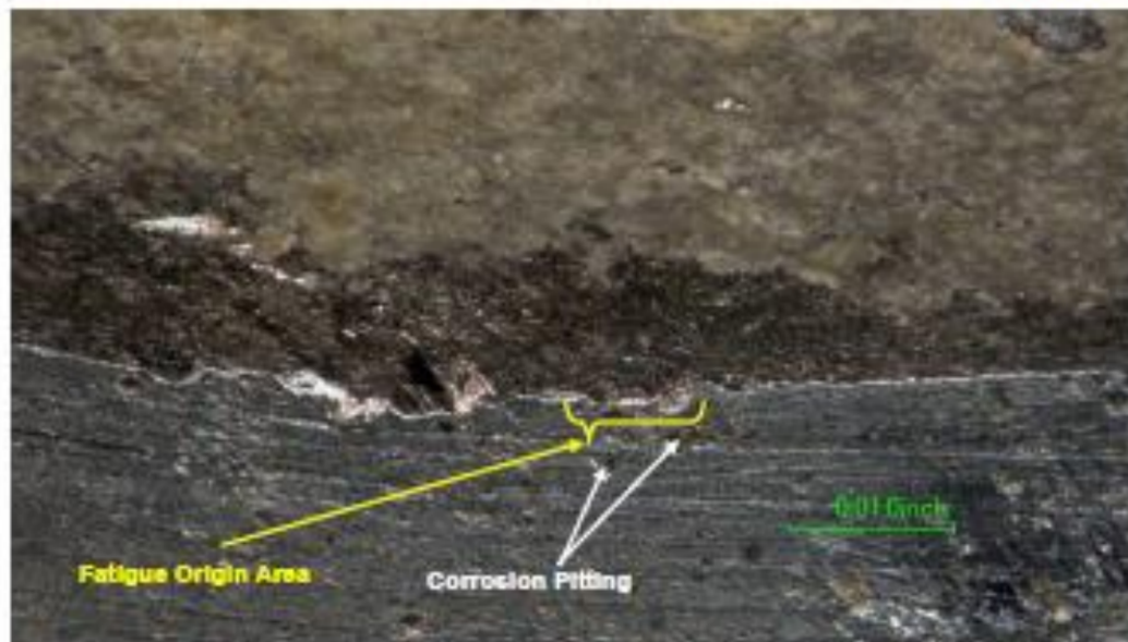
Figure 5: High magnification optical image showing fatigue origin location tilted to show the condition of the clevis surface.
