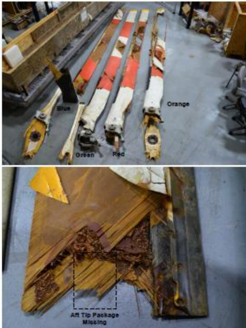
Figure 8: Overview of the blades (top image). The aft tip weight package was missing from the Blue blade (bottom image)
